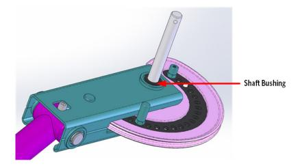
5. Flip the arm assembly over and remove the bottom shaft cap using the same procedure that was used in step 3 to remove the top cap. Use the Tri-Flow PTFE to lubricate the shaft at the edge of the IGUS bushing flange. Rotate the shaft by hand to work the lubricant into the joint. **See Diagram 8**.
