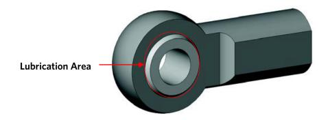
Check cable rod ends to make sure the shoulder bolts are secure. If cable rod ends are noisy, lubricate them with a silicone spray lubricant or Lithium grease. Apply the lubricant onto the joint where the spherical portion is enclosed in the outer housing, as shown in **Diagram 1**. Wipe off any excess lubricant with a cloth.
