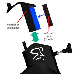
Add a coating of the "Lucas Red "N" Tacky #2 Grease" to the threads of both the handlebar and seat post height adjustment pop-pin bolt threads.
