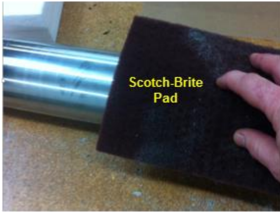
Use a Scotch-Brite pad to clean surface
